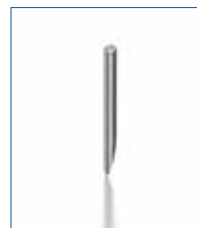
Stylus tip 33 mm Order no.: 101-011-330 made of carbide, \varnothing 3.5 mm / R: 25 \mu m / A: 12° with optaGold coating
