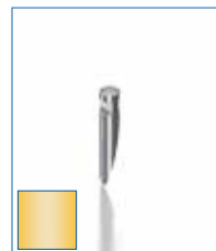
Stylus tip 59.5 mm Order no.: 101-010-595 made of carbide, \varnothing 3.5 mm / R: 25 \mu m / A: 12°
